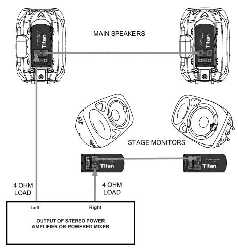
**NOTE**: This configuration represents a 4 ohm load to each output channel of the amplifier.
